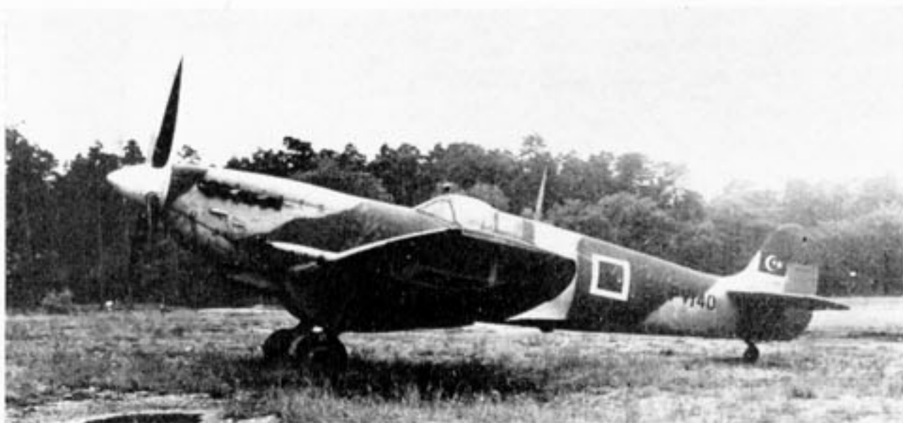
The Turkish Air Force had at least 44 Spitfire L.F. Mk. IXEs supplied to them in 1945. This example retains its R.A.F. serial PV140 and long-range tank. (Photo: J. D. R. Rawlings)
