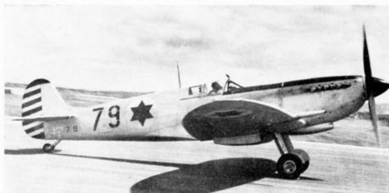
A superb shot of an I.D.F./A.F. Spitfire L.F. Mk. IX E taxiing. Note miniature repeat serial 79 and national marking between large 7 and 9.
