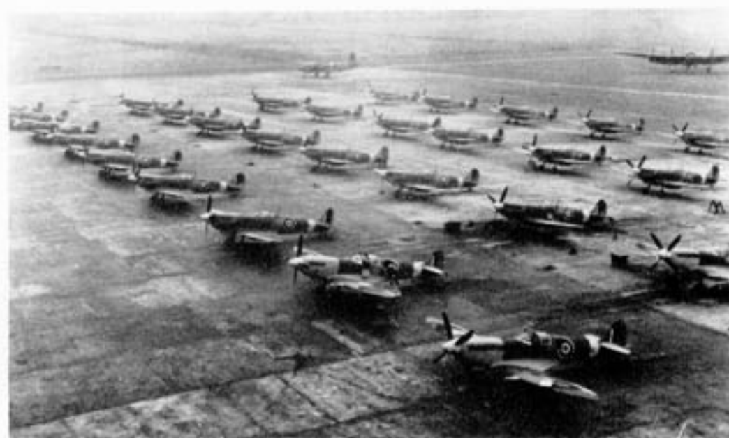
Spitfire Mk. IX Es awaiting collection at the Castle Bromwich factory in 1944. Aircraft in the front row include (right to left): NH432, NH311, NH419, NH45 and NH425. Some cowlings, wing fillets, ailerons and tailplanes require final camouflage. (Photo: via Bruce Robertson)
