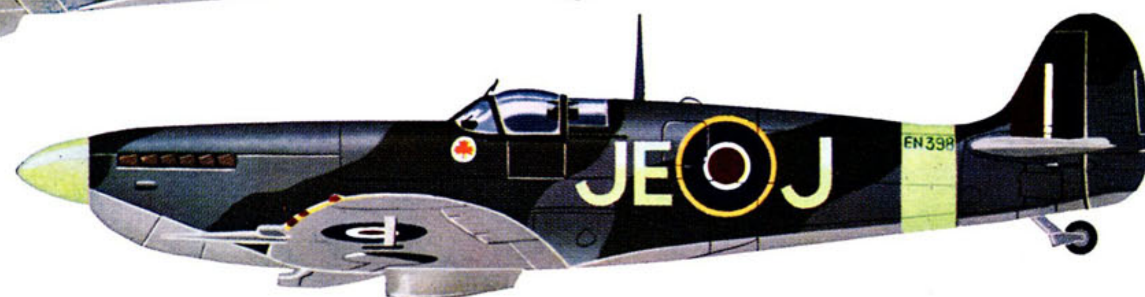
RR246 of No. 43 (F) Squadron "A" Flight, circa 1945. "B" Flight had blue codes and aircraft letter. Type C upper wing roundel. Sky band painted out. On some aircraft under-surface grey was used for this purpose.
